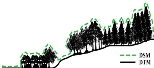
**Gambar 2 Digital Terrain Model (DTM)**
